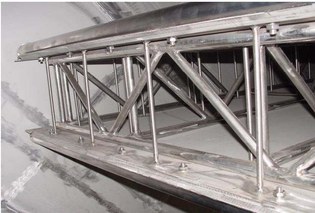
The lattice structure reinforced blade with cardinally attached free floating cover plates remains free of distortions when subjected to high and rapidly changing temperatures. High temperature gas flows continuously through the blade's latticed support structure, all parts of which heat up evenly. The design of the lattice structure is based upon the "finite element" method. In this connection, please refer to our publication "**TECHNOLOGY 6**"
