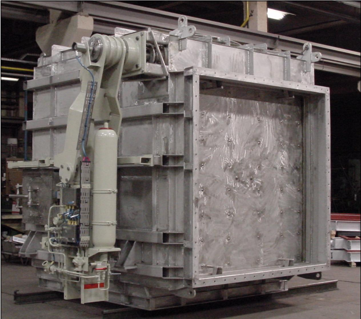
**RAUMAG – JANICH** obtained an order from **ALSTOM Energy Systems**, UK for the supply of a diverter damper, ND 2100 x 2100 mm, for an off – shore gasturbine plant in Denmark.
