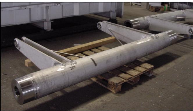
*The picture on the left shows a diverter drive shaft with toggle levers.*
