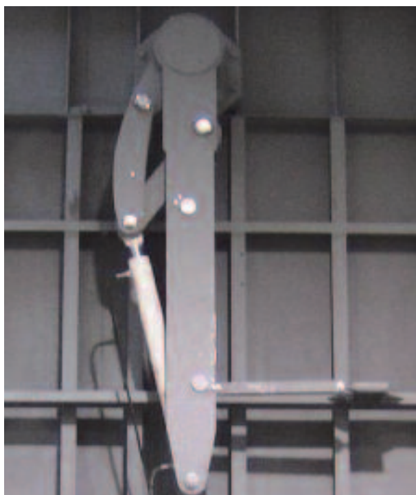
Picture below: dual toggle lever actuation arrangement for a DIVERTER, ND 5600 x 5600 mm
