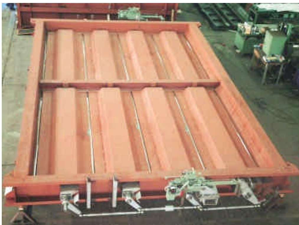
Louver damper, ND 8220 x 5300 mm, for a FGD plant, designed with profiled blades and NICROFLEX-MLO type seals.
