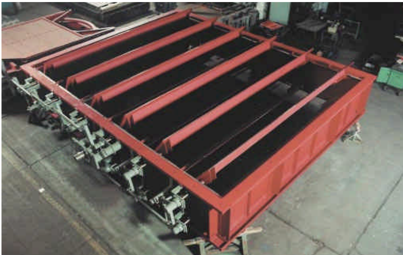
△ Double louver damper, ND 6780 x 5390 mm , for FGD plant. With seal air, 100% gastight in terms of UVV regulations. Seals are of the NICROFLEX-HIPERFORM, DBP, type.
