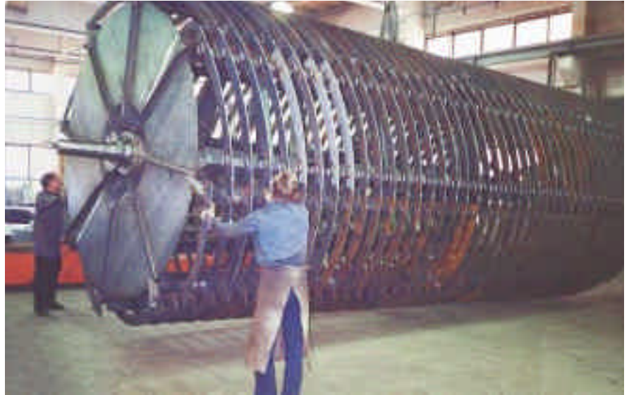
Picture above: Rotor of a cement cooler, 3200 mm dia., length 8500 mm
