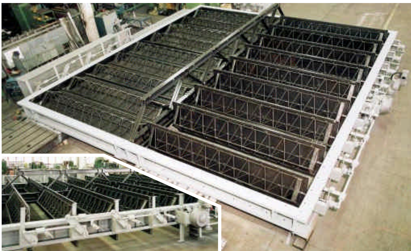
▽ Louver damper, ND 9000 x 10000 mm , for the gastight isolation of a DeNOx catalytic reactor. The new, patented, lattice supported single shell damper blades, DBP, minimise the pressure drop across the open damper and no distortion occurs when exposed to high temperatures.
